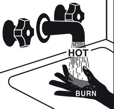
This water heater can make water hot enough to cause severe burns instantly, resulting in severe injury or death. Be careful to have children, disabled and elderly not exposed to scald risk. Before setting temperature at water heater, see instruction manual. Test water temperature before bathing or showering. Refer to manual for temperature limiting valves reference.
