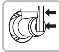
Lower lever carefully until water flows from drain line.
