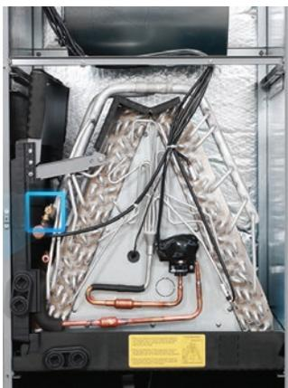
◀ The indoor coils are factory charged with nitrogen to ensure a clean, dry and contaminant free system that is ready for installation. An installed check valve can be used to ensure the integrity of the coil.
